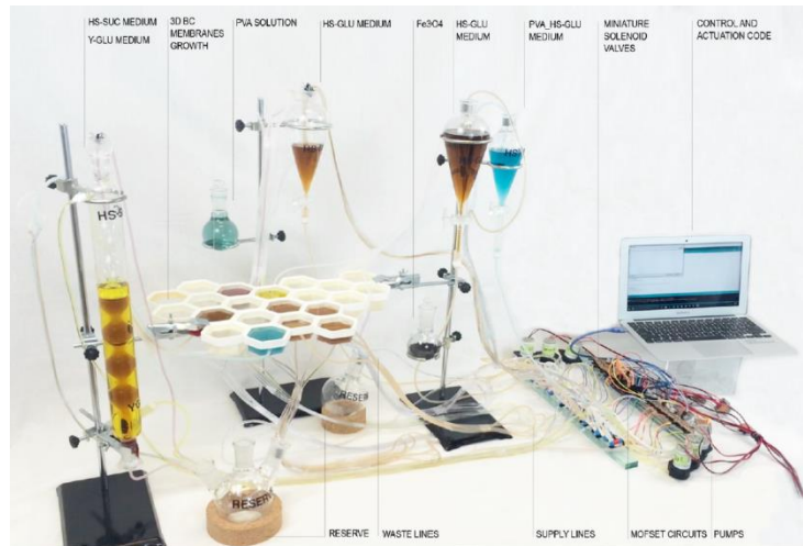
Figure 3: Setup for Zolotovskiy's growth process (Zolotovskiy)
