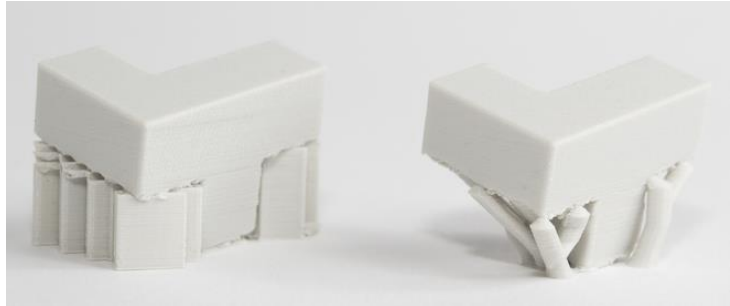
Figure 5: Accordion and tree supports (Cain)
